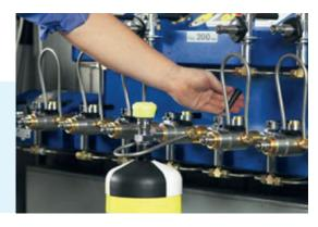
OUR BREATHING AIR ADAPTERS WERE DEVELOPED FOR FAST CONNECTION OF BREATHING AIR CYLINDERS.
